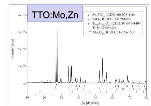
Crystal structure of SnO<sub>2</sub>/TiO<sub>2</sub>-based composite ceramics confirmed; -major crystal phase indexed as  $Sn_{0.2}Ti_{0.8}O_2$  (ICDD card no. 01-070-4404), -impurity related XRD peaks indicate traces of SnO<sub>2</sub> (ICDD card no. 01-079-6889) in TTO-Mo and TTO-Mo,Zn; Zn<sub>2</sub>TiO<sub>4</sub> (ICDD card no. 00-025-1164) in TTO-Mo,Zn; and Mo<sub>9</sub>O<sub>26</sub> (ICDD card no. 01-073-1536) in TTO-Mo,Zn).
